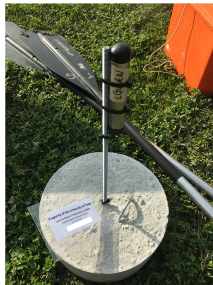
Figure C.1. Sensor mount and installation setup
