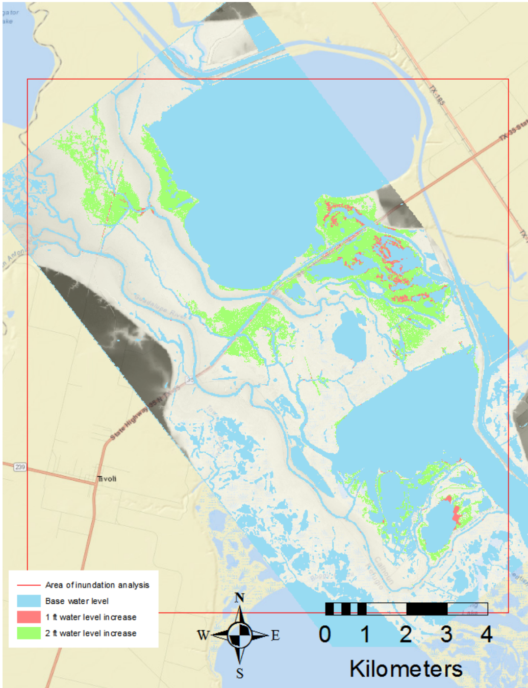
Figure 9. Inundation levels of 1-2 ft above base estimated water level
